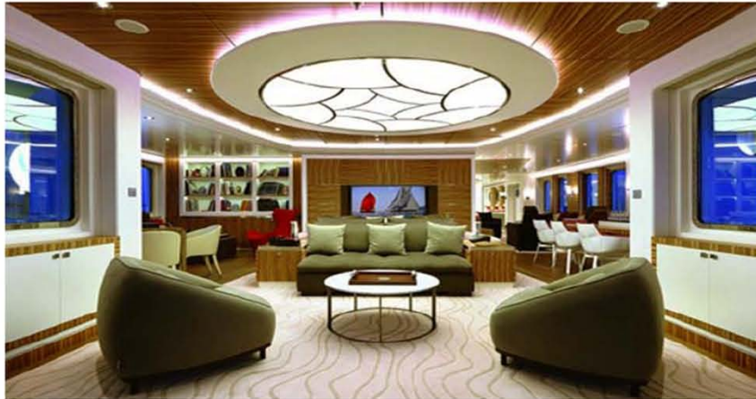
Zebrano and oak veneers give contrast throughout the interior. Wood is kept to a minimum, with man-made material for exterior decks rather than the usual teak.
